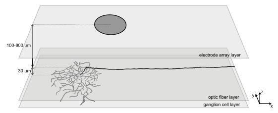
Fig. 1: Spatial configuration of the computational model of epiretinal electrical stimulation. A simulated mouse ganglion cell occupied the ganglion cell layer, with its axon extending into the optic fiber layer, and a simulated disk electrode ( $200 \,\mu m$  diamater) placed at varying distances ( $100 - 800 \,\mu m$ ) above that.
