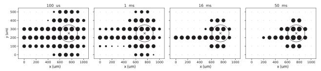
Fig. 4: Effect of stimulus pulse duration on ganglion cell responses. Large open circle: epiretinal disk electrode. Small dots: number of spikes emitted by a cell at a particular location (largest dot: 21 spikes). Optic disc lies to the right of each image.
