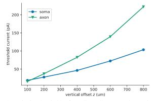
Fig. 3: Excitation thresholds of ganglion cell somas and axons in the population model for an epiretinal disk electrode (200  $\mu m$  diameter) located at varying vertical offsets (z).
