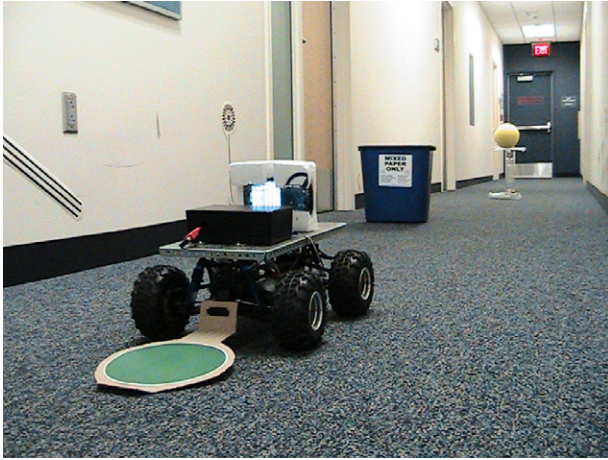
Fig. 1. “Le Carl” Android based robot, which was constructed from the chassis of an R/C car. The task of the robot was to navigate to a visually salient target (bright yellow foam ball) while avoiding an obstacle (blue recycle bin) along the way. The robot’s position throughout the task was recorded by an overhead camera that tracked the position of the green marker. (For interpretation of the references to color in this figure legend, the reader is referred to the web version of this article.)
